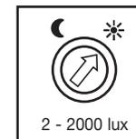
The sensor's response threshold can be infinitely varied from 2 – 2000 lux.
